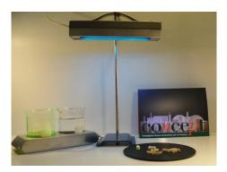
This technique is based on capillary phenomenon and on specific physical characteristics of liquids such as surface tension and viscosity in order to detect surface defects on material which are not porous on surface, like sintered Zirconia, alloys, etc.
